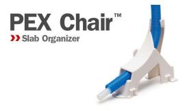
features include a rebar receiver for ground staking, as well as height adjustment for pre-cast deck over pours. The angled design and hook feature at the top of the unit makes it easy to install PEX without kinking and holds the tube vertically in place through the completion of the concrete pour.
