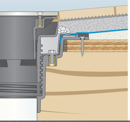
In a traditional shower pan application with sheet pan liner, the Coring Sleeve allows for a faster, easier installation of the secondary mortar bed.
