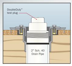
Set drain body and fasten to sub floor. Connect drain pipe and test using the DoubleDuty™ test plug (included).
