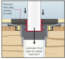
Attach gasket and connect tailpiece to the tub outlet. Align with drain body and lower tub into place. The gasket pushes in to seal inside the 2" drain pipe
