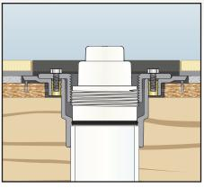
Install tile/flooring as desired. The test plug can remain in place to protect drain line from construction debris.
