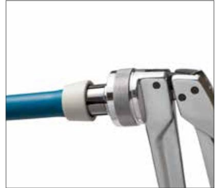
**3.** Using pipe expander, expand ring fully. Repeat expansions, rotating expander 1/8-turn between expansions.
