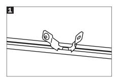
**1.** Separate clamp and place in bracket.
