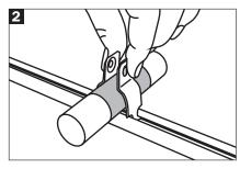
**2.** Wrap copper with 10-mil tape and install between 2 halves.
