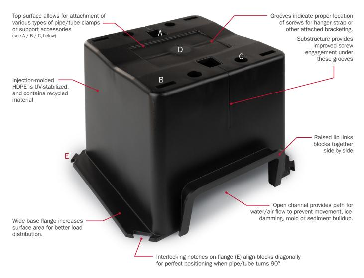
A: Unique openings (2) allow use of inverted TD+ Universal Clamp (550-2111) to fasten 1/2" CTS -2" IPS
