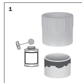
Glue adapter to pipe using appropriate solvent cement.
