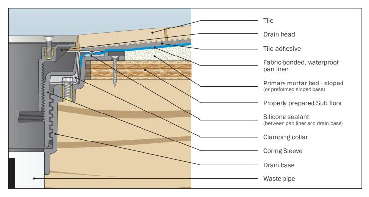
1 Fabric-bonded waterproof pan liner should be certified/approved, and conform to ANSI A118.10
