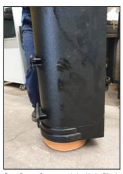
On a flat surface, stand the HydroBlock section up vertically and using the weight of the section, slowly lower onto the pipe connector
