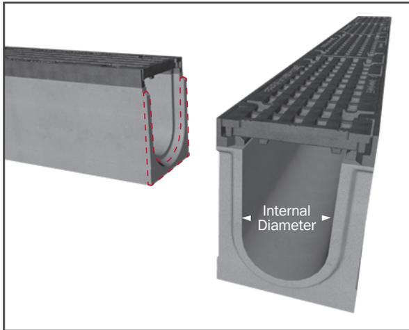
Confirm channels are the same height and internal diameter. Remove flanged end (approx 0.3") from "branch" section if necessary.
