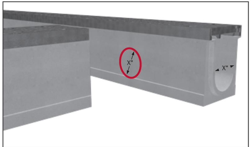
Determine location for branch and cut/drill an opening into "trunk" section that matches the internal diameter. The bottom of the opening hole should align with the bottom of the channel in the trunk section.
