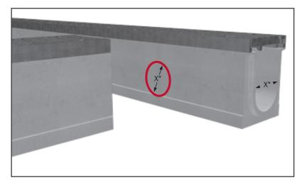
Determine location for branch and cut/drill an opening into "trunk" section that matches the internal diameter. The bottom of the opening hole should align with the bottom of the channel in the trunk section.
