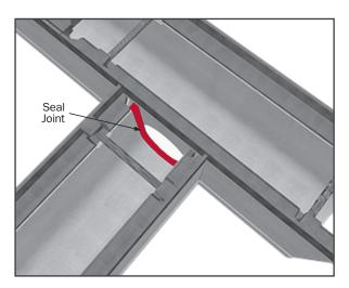
Align the branch section with the opening hole and butt the branch as closely as possible against the side wall of the trunk section. Use a one-part epoxy to seal the joint between the branch and trunk sections.
