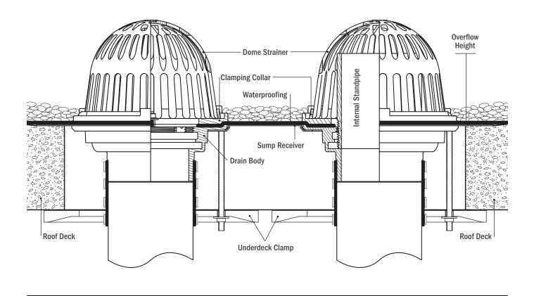
**STEP 1:** Refer to local code requirements for emergency/secondary overflow roof drainage. Local codes vary but it is recommended to provide a drain to overflow ratio of 1 to 1. Roof drains shall be installed only in areas where waterproofing material is utilized.
