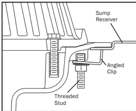
Set drain on flat surface with outlet facing up.
