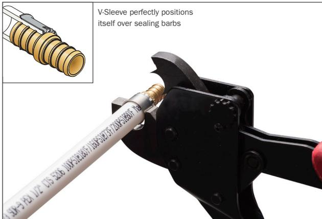
4. Assure sleeve is fully installed onto end of tube and fitting is inserted fully into tube end. Compress tool perpendicular to tube. Compress only once.
