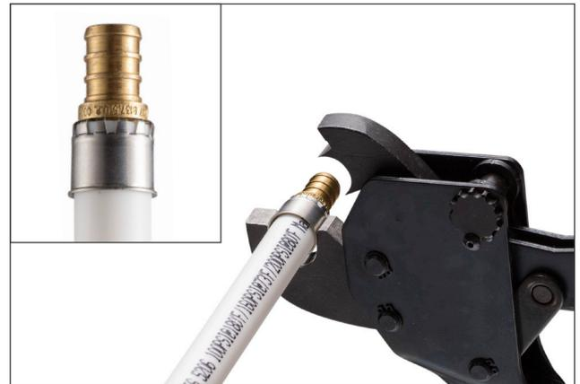
5. Remove any defective connections. Use a gauge to assure a proper joint. Test all completed joints.
