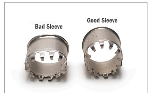
Always check sleeves before use. Creased or bent sleeves should never be installed.
