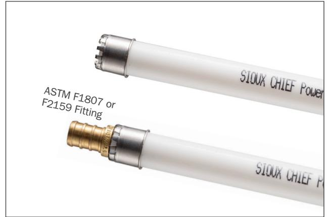
2. Install V-Sleeve onto OD of tube with notched side towards tube end. Install fitting fully into tube. Visually confirm tube is fully inserted through V-Sleeve notches.
