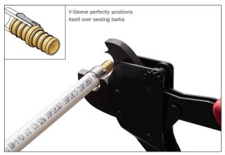
4. Assure sleeve is fully installed onto end of tube and fitting is inserted fully into tube end. Compress tool perpendicular to tube. Compress only once.
