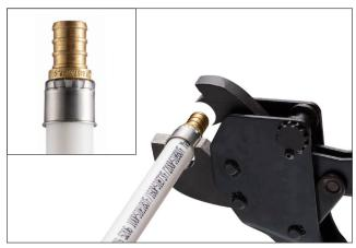
5. Remove any defective connections. Use a gauge to assure a proper joint. Test all completed joints.
