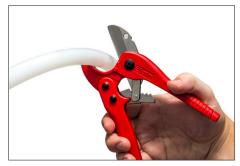
1. Cut tube at 90-degrees. Do not crush OD of tubing with cutters. Hint: Slightly rotate cutter during blade engagement.
