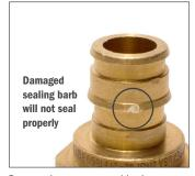
Damaged, cut or grooved barb on fitting.
