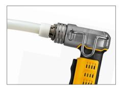
3. Using expander tool, expand sleeve fully. If using a manual tool, expand slowly and repeat expansions, rotating expander 1/8-turn between expansions. Forcing the tube onto the expansion head and/or expanding too quickly can damage the tubing and sleeve, and require rework.
