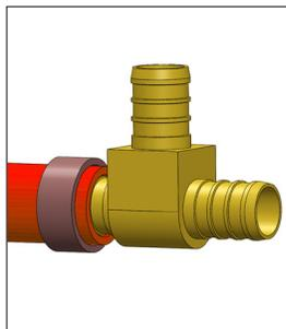
Fitting not inserted completely into tube end.
