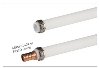
2. Install ASTM F2098 stainless steel cinch clamp onto OD of tube. Install fitting fully into tube.
