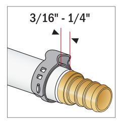
1. Position clamp between 3/16" and 1/4" from tube end to ensure coverage of both sealing barbs.
