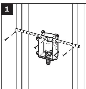
Slide bracket into top track and secure bracket to studs
