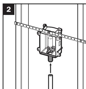
Connect supply line according to industry standards. Open valves before any soldering
