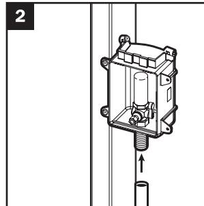
Connect supply line according to industry standards. Open valves before any soldering
