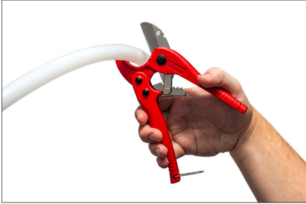
1. Cut tube at 90-degrees. Do not crush OD of tubing with cutters. Hint: Slightly rotate cutter during blade engagement.
