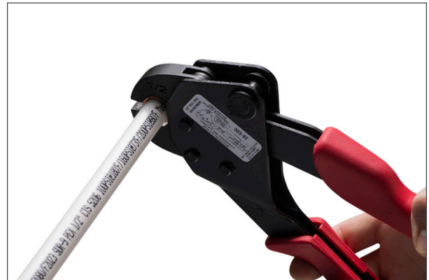
4. Compress tool perpendicular to tube. Compress only once. Remove defective connections. Use a gauge to assure a proper joint. Test all completed joints.
