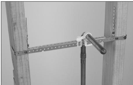
For narrow stud bays, break perforation at the corner of the bracket to best fit the opening.
