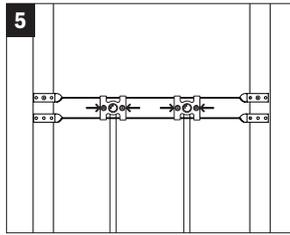
5 Tighten each screw on each block to secure stub out and prevent horizontal movement.
