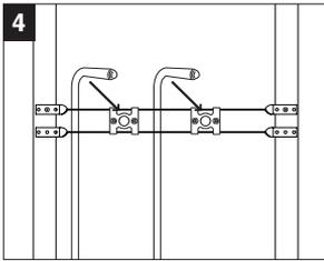
4 Install stub outs or stub out elbows.
