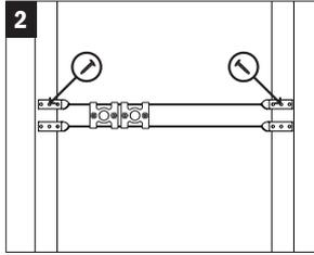
2 Secure top bracket to studs on each side of stud bay. Do NOT secure bottom bracket yet.
