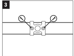
Insert one #6 × 1" screw in each hole and tighten so the blocks are secured together, but they are able to slide back and forth along the brackets.
