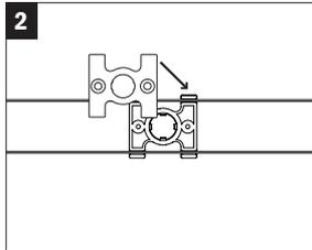
Position the female block directly on top of the male block.
