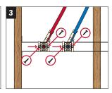
Slide plastic elbow block assembly to desired stub out location. Insert two screws into each block and tighten. Tightening screws prevents lateral movement of blocks on brackets and prevents elbow from swiveling.
