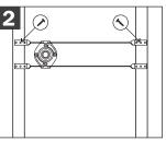
Secure top bracket to face of stud bay at desired position for shower arm stub out.
