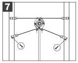
Secure ends of bottom bracket to studs.
