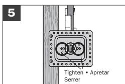
Complete the installation by tightening all screws to prevent movement.
