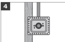
Working from the back, push  $\frac{1}{2}$ " PEX through LockBlock and plate. Do Not kink the tube.
