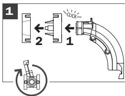
Snap elbow into back of LockBlock until it clicks. Snap the two halves of LockBlock together. The elbow should spin freely.
