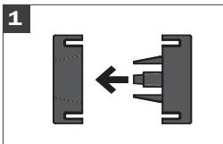
Snap the two halves of LockBlock together.
