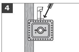
Working from the back, push  $\frac{1}{2}$ " PEX through LockBlock and plate. Carefully secure tube in bend support. Do Not kink the tube.
