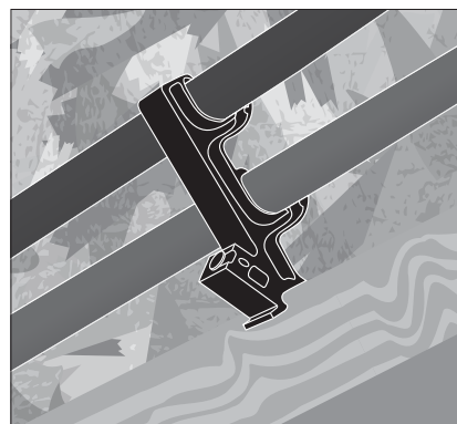
Completed Installation when installed on edge of engineered wood joist flange
