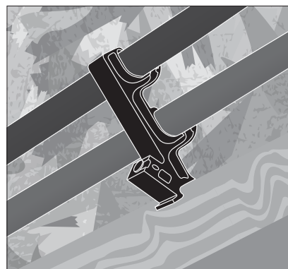
Completed Installation when installed on edge of engineered wood joist flange
