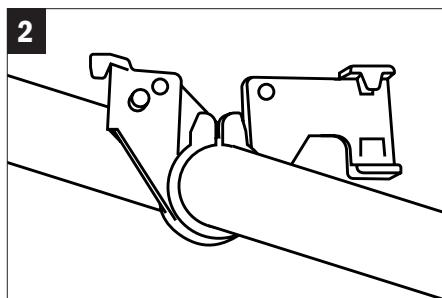
Insert tube into SimpleStrap clamp.
