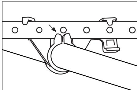
Note: The ears of the clamp should lock on the front of the bracket.
