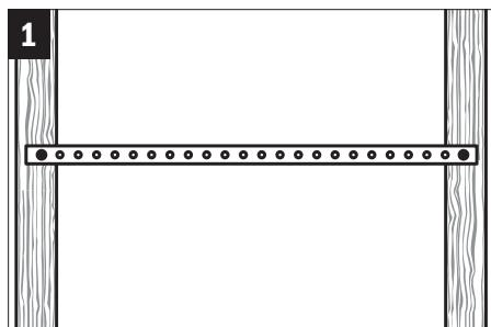
Attach flat Support Bracket to studs using nails or screws.
