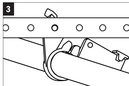
Align tooth through one of the bracket holes, twist clamp counterclockwise, and click tabs onto bracket.
